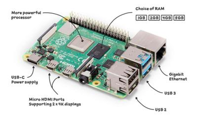
The core board needs to be accessorized to function with a case and power supply. A HDMI monitor and USB mouse / keyboard are for initial setup and configuration although once you've loaded the operating system to the device you can connect to it wirelessly from your computer or tablet via a built-in wireless hub. The board also includes a gigabit Ethernet port for direct connection to your network, which I tend to prefer over wireless unless out in the field.
