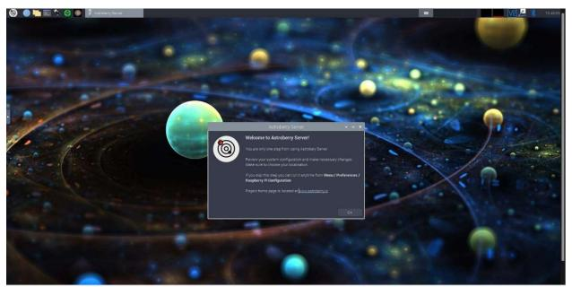
Starting up with an AstroBerry image on your MicroSD card or SSD will boot the AstroBerry operating system and present you with an operating system screen similar to Windows as shown above. The OS runs the Raspberry Pi configuration utility that allows you to change the configuration of your Raspberry Pi – for now, you can just click on ok to close the utility (it can always be run from the menu at top left under Preferences/Raspberry Pi Configuration.
