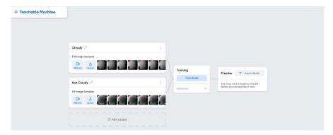
I uploaded each set of images via drag and drop to the TM web set to create my two classes of images, as seen above. Next I clicked Train Model, and a minute or two later, it presented me with a completed model I could export and download, as well as a test panel I could drop image files to and see what the model produced for these images.
